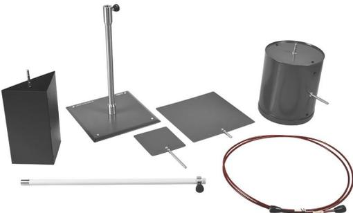
The RCS Demonstration Accessories kit contains all the accessories required to measure the relative RCS pattern of targets using the ATMS. It includes targets of various shapes (small and large metal plates, cylinder, and prism-shaped target), a 2 m SMA cable, a fixed antenna support, and an antenna mounting pole.
