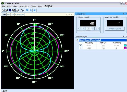
Figure 1. The E-plane and the H-plane patterns are acquired separately. These patterns can be plotted on a polar graph (as shown in figure) or a Cartesian graph (see Figure 2).
