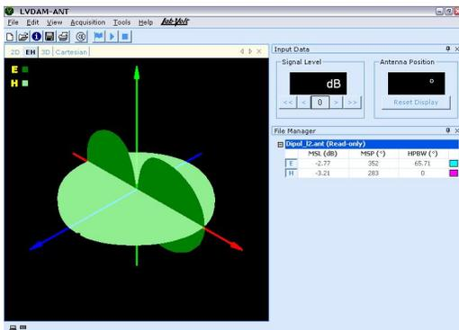
Figure 3. The acquired E- and H-plane patterns can be displayed simultaneously on a tri-dimensional (3D) display (shown in figure: dipole antenna pattern).
