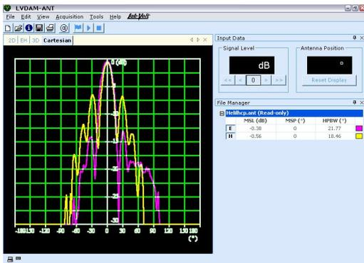
Figure 2. E- and H-plane patterns of an helical antenna plotted on a Cartesian coordinate graph.
