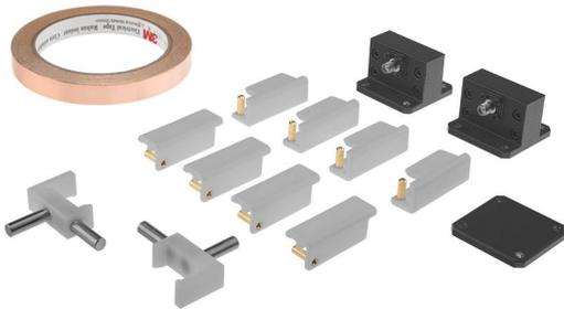
The Waveguide Accessories kit contains the accessories required when using the horn- and waveguide-type antennas of the ATMS. The kit includes quick-lock fasteners, waveguide-to-coaxial cable adapters (SMA connector), a waveguide plastic holder, a waveguide short-circuit, and copper tape to modify the characteristics of the slotted waveguide and patch antennas.
