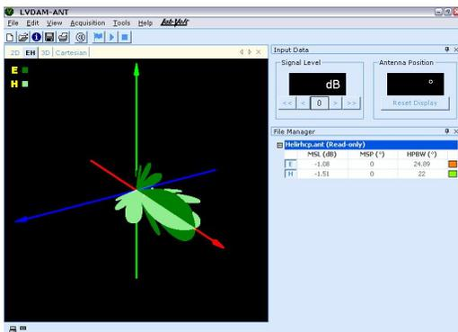
Figure 4. The acquired E- and H-plane patterns can be displayed simultaneously on a tri-dimensional (3D) display (shown in figure: helical antenna pattern).
