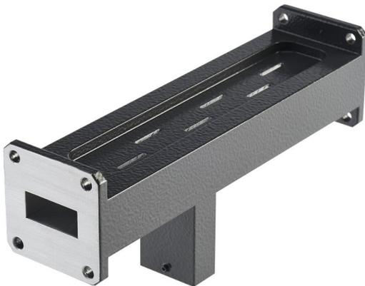
The Slotted-Waveguide Antenna is a light-weight, small-size WR90 waveguide-type slotted antenna. The slot antenna is of the "standing wave array" type. The array is terminated by a short circuit at the end of the waveguide.
