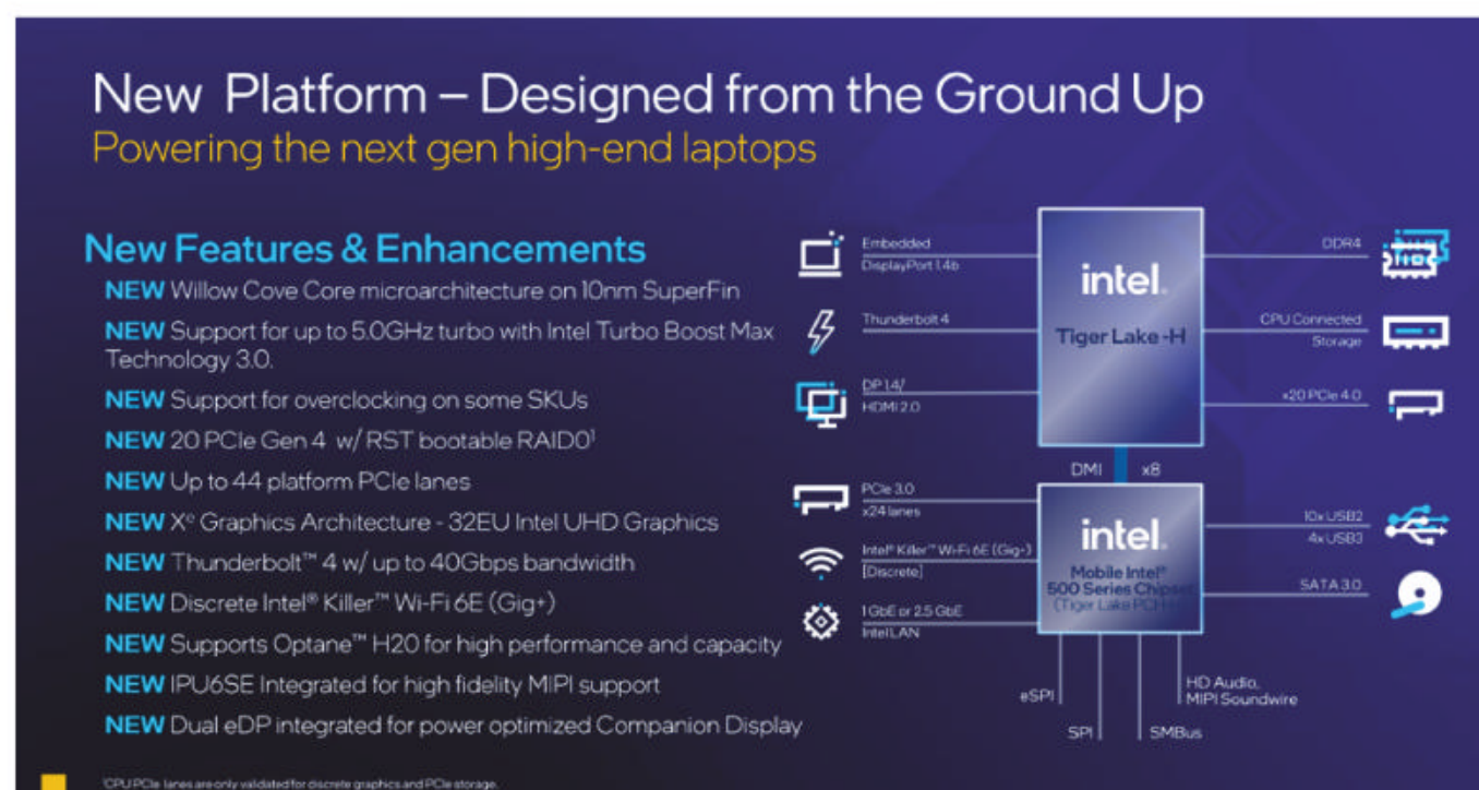
A summary of the improvements Intel has added to its mobile 11th-gen Core platform, code-named Tiger Lake H.
