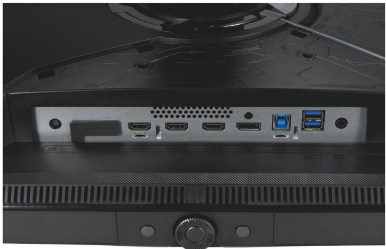
You get DisplayPort, three HDMI ports, and plenty of USB ports. That jog dial lets you easily change monitor settings.
