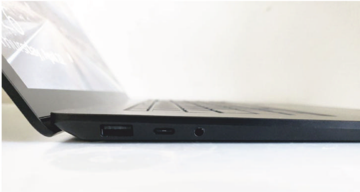
The Surface Laptop 4's port arrangement is minimal: USB-C, USB-A, and a headphone jack.
