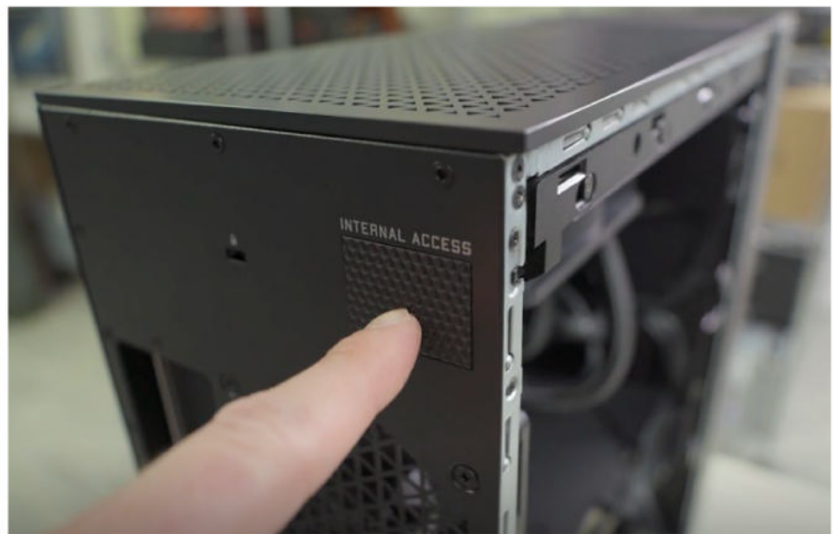
Getting into the HP Omen 30L's case is a snap—just press the Internal Access button.
