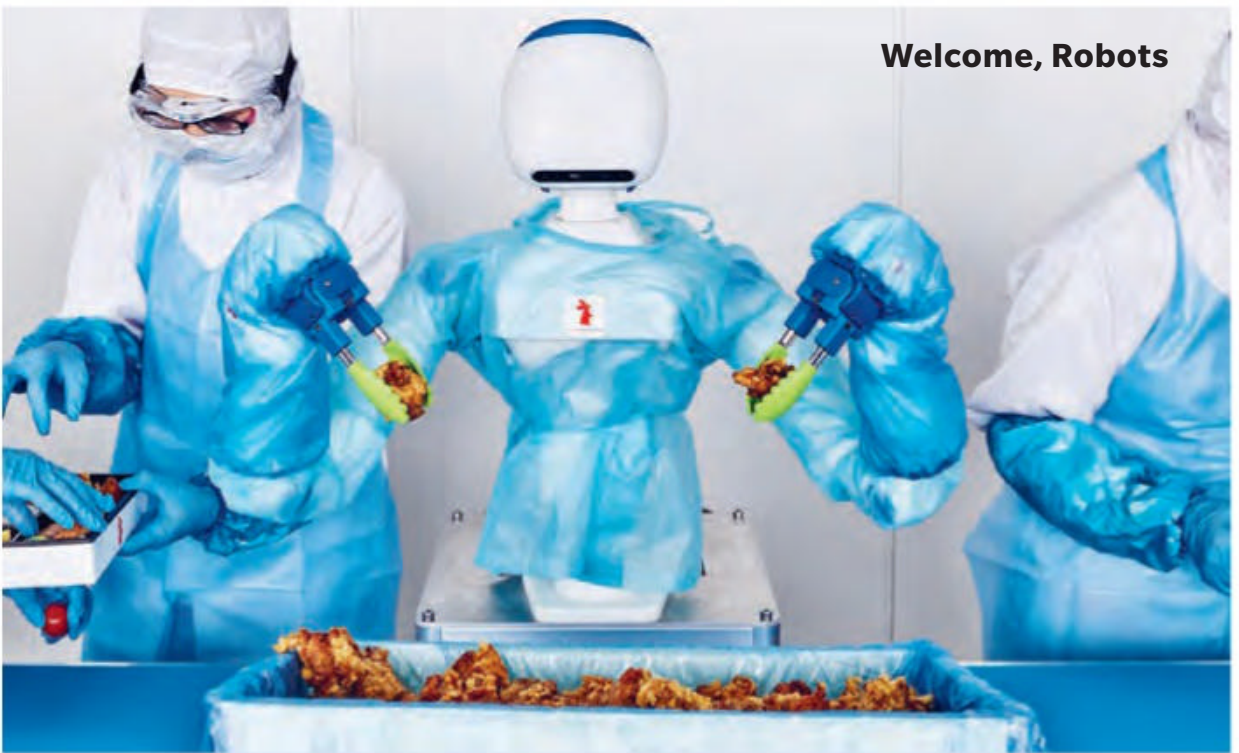
Foodly, a collaborative robot, or cobot, developed by RT Corporation, uses advanced vision, algorithms and a grasping hand to place pieces of chicken in a bento box
