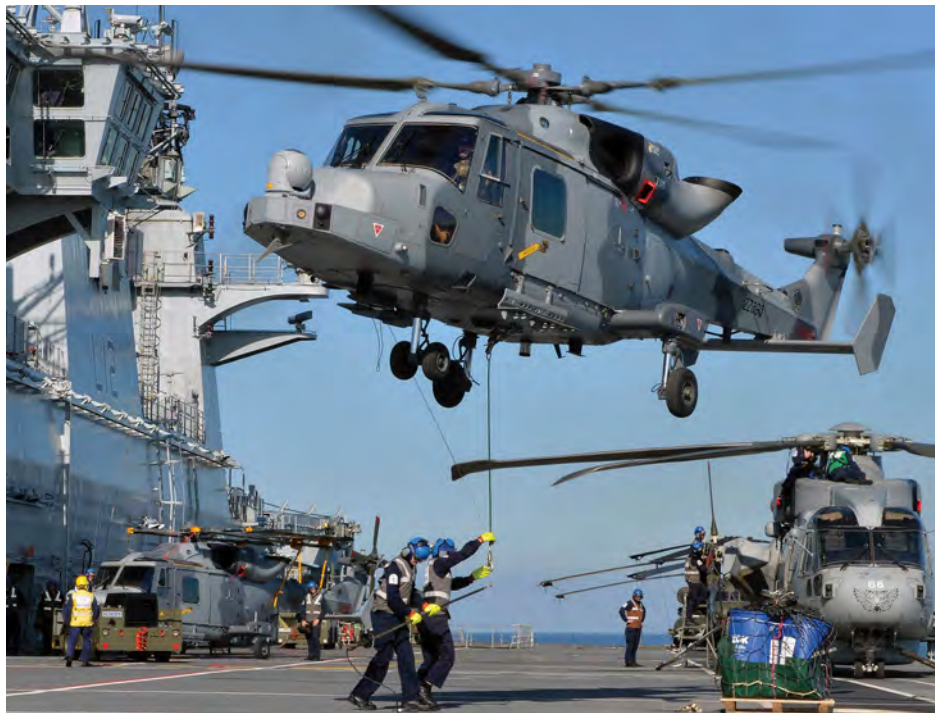
Above: Deck crew attach a static line to a Wildcat landing on HMS Ocean during Exercise Trident Juncture 2015 LPhoto Des Wade/MOD Crown Copyright 2015
