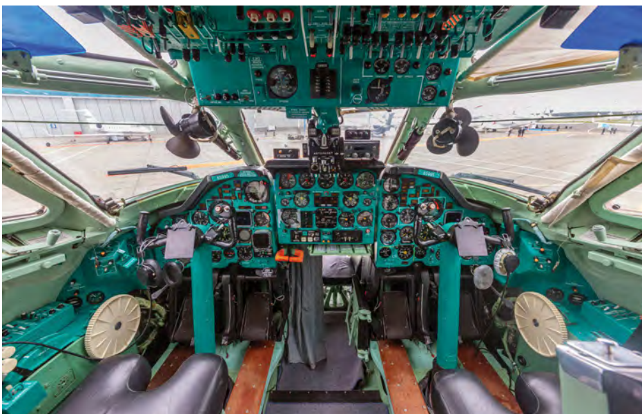
The typically Soviet-era cockpit of RA-65995, a Tu-134A-3 of Russian charter operator Kosmos Airlines. Note the crawl-way between the pilots leading to the navigator's position in the nose
