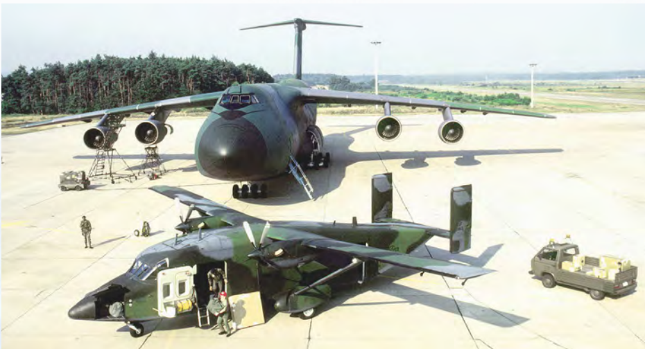
Below: Inter-theatre C-5A Galaxy and intra-theatre C-23A Sherpa on the ground at Zweibrücken AB. The Sherpa's double-size side cargo door is open in this shot USAF/CMSgt Don Sutherland
