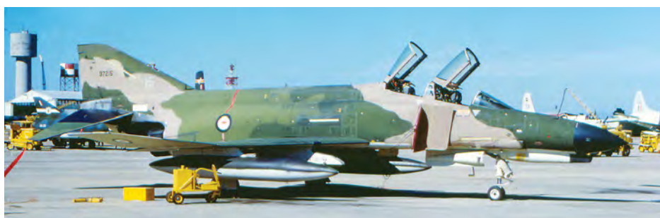
Phantom s/n 7215 showing the standard USAF Southeast Asia camouflage scheme of the time, applied to all RAAF Phantoms. Australia's F-4Es were all new aircraft from Production Block 43, built in mid-1970 Robert Wiseman
