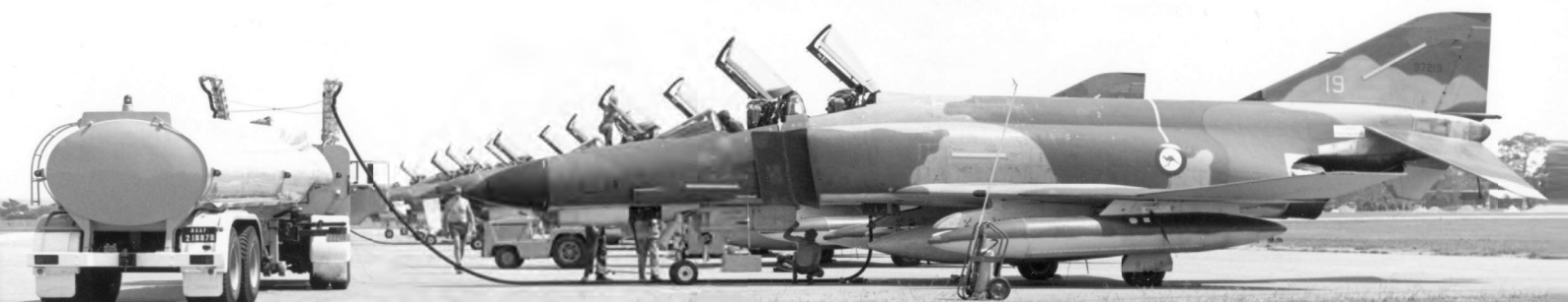
Half a dozen 'thirsty' Phantoms line up for a drink at Amberley. The F-4E's internal fuel capacity was nearly 1,850 US gal and external tanks could add another 1,321 US gal to this amount RAAF
