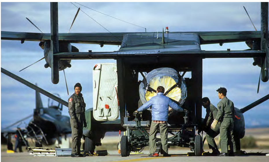
An essential requirement for the C-23A's selection was the capability to carry fighter engines. Here, an F-16 powerplant is loaded at Zaragoza AB USAF/SSgt Fernando Serna
