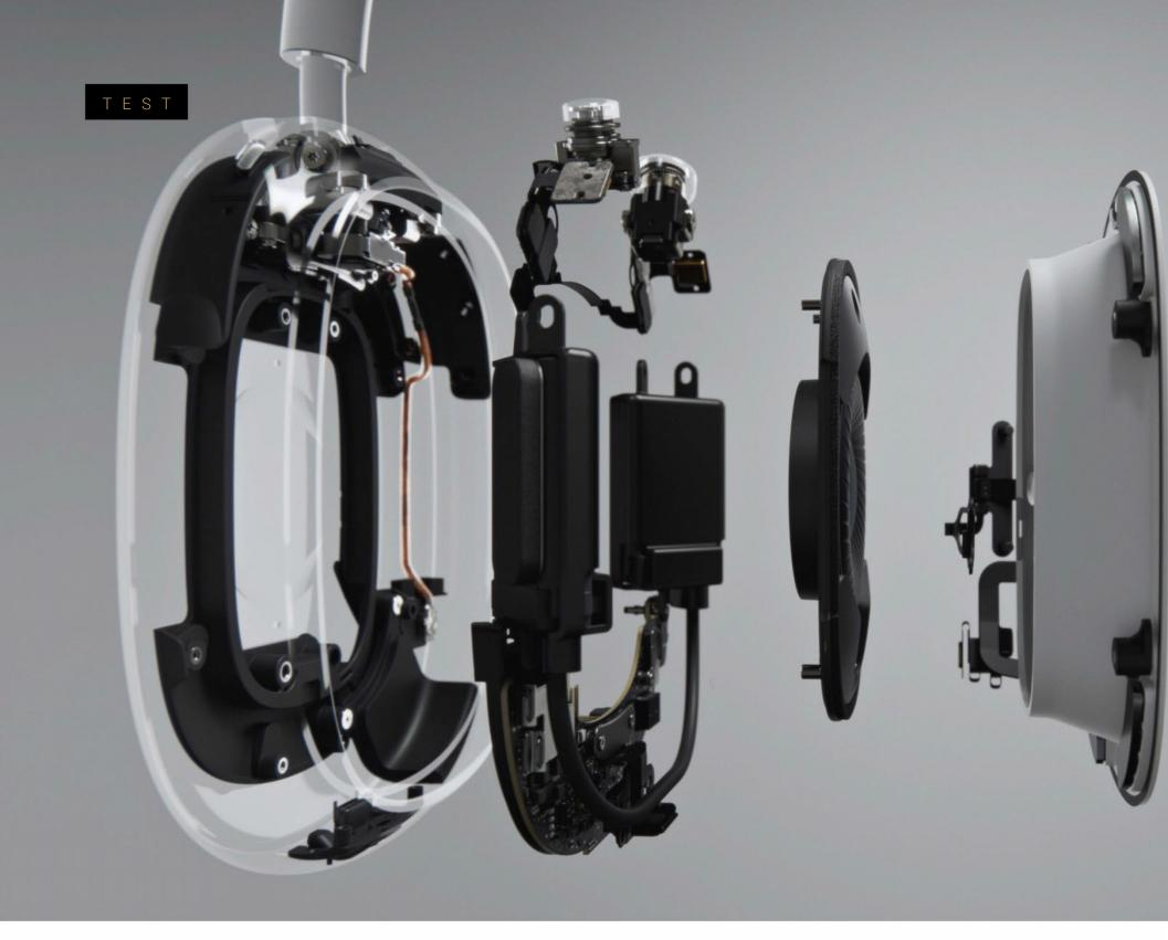
the internal mic and H1 chips to analyse sound going to your ears and adjusts the driver's frequency response to match its target tuning. It does this to compensate for variances in fit and seal so that it can deliver a consistent sound regardless of your anatomy.
