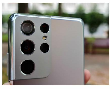
The quad-rear camera S21 Ultra swapped out a 3D depth sensor for a second telephoto lens and Laser AutoFocus sensor.
