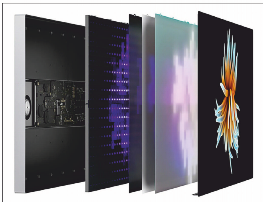
The Pro Display XDR has hundreds of LED backlights, but not enough to be truly called a Mini LED display.
