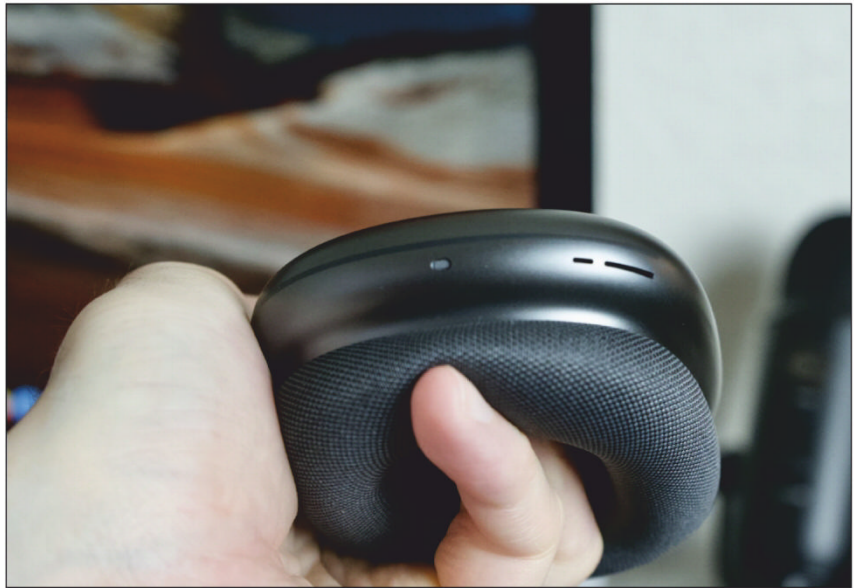
The AirPods Max have nine microphones, behind tiny slits all around the edges.
