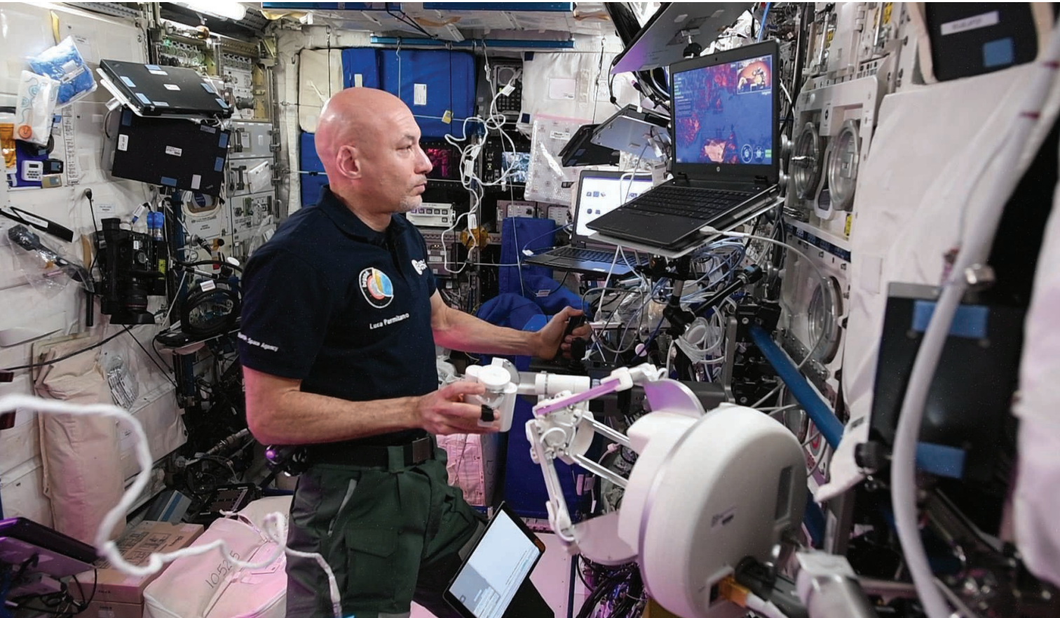
From space ESA astronaut Luca Parmitano uses the haptic platform to control a robot manipulator ©2019 ESA
