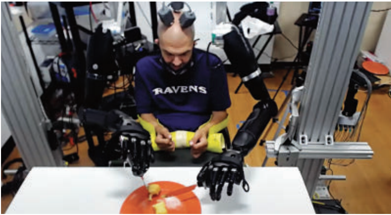
Robert “Buz” Chmielewski, who has had quadriplegia since his teens, uses brain signals to feed himself some cake. Via electrodes implanted in both sides of his brain, he controls two robotic arms: One manipulates the knife and the other holds the fork.
