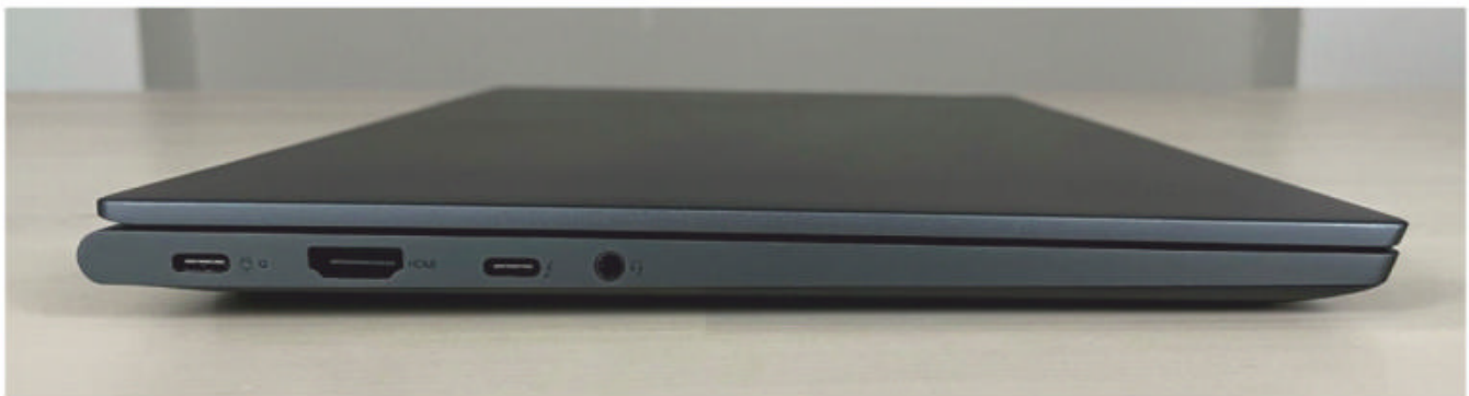
The left side of the Lenovo IdeaPad 7 features a Thunderbolt 3 port, a full HDMI port, a combo audio jack, and a USB-C power port.
