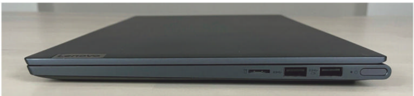
A pair of USB SuperSpeed 5Gbps Type-A ports sit on the right side, along with a microSD slot. A fingerprint reader is embedded in the power button.
