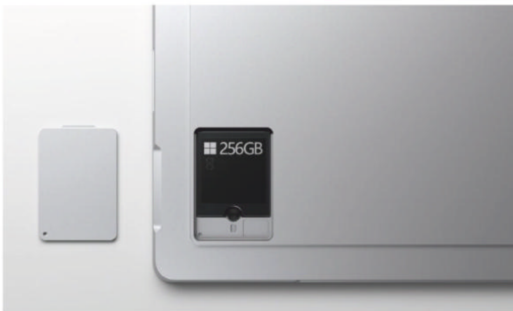
The Surface Pro 7 adds an SSD drawer, and the ability to swap out the SSD inside.
