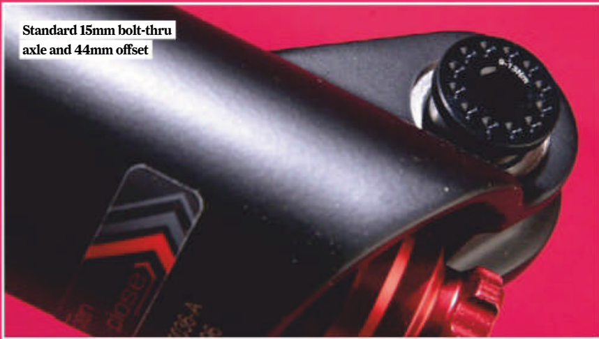
Extended fork crown boosts stiffness
