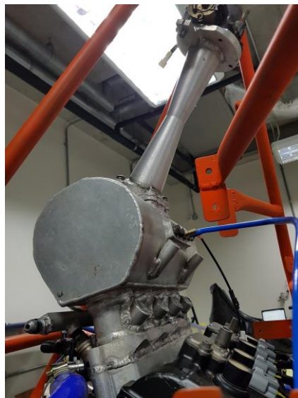
Figure 2. Picture of the Old Air intake in the chassis of TR16
