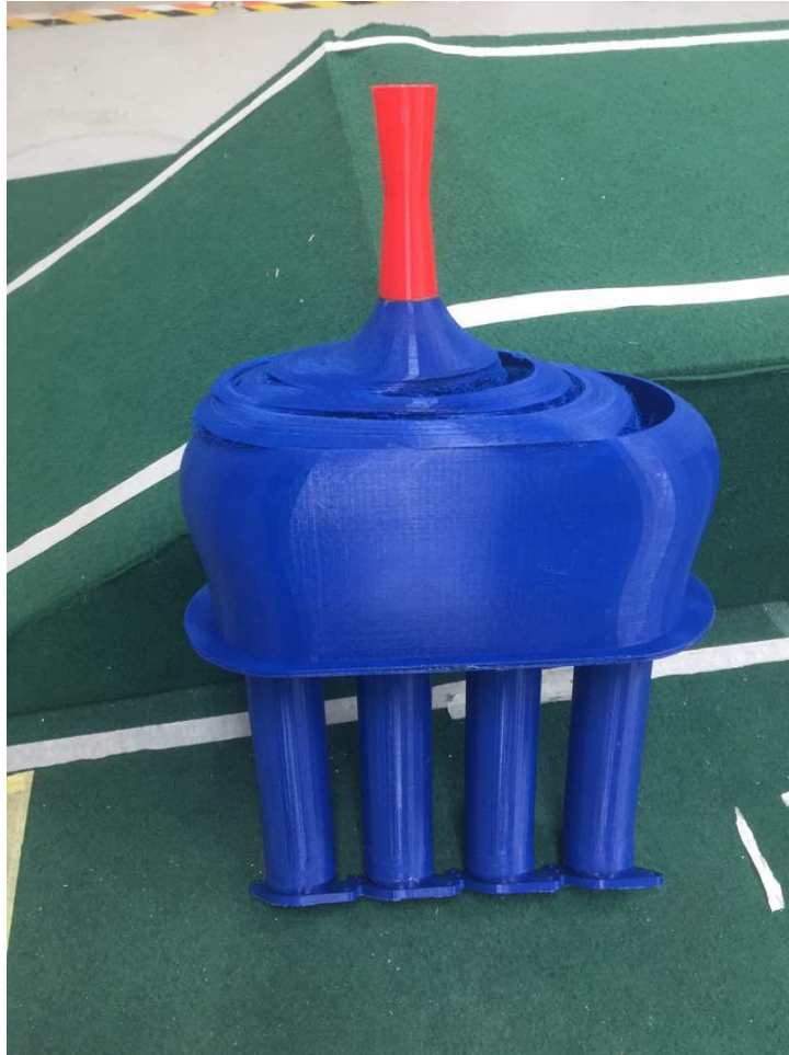
The top part of the plenum is displaced from the rest of the intake
