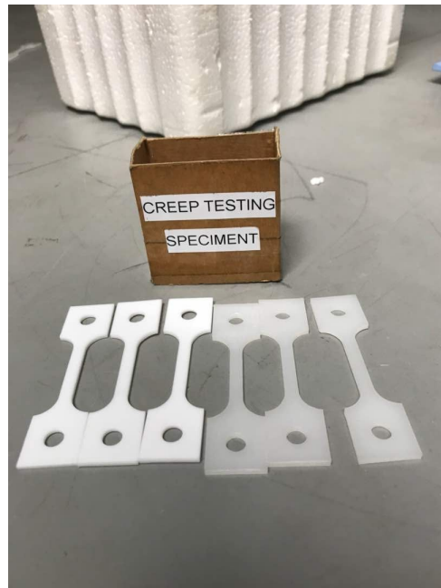
Figure 4. The teflon and PDFE specimens for the experiment
