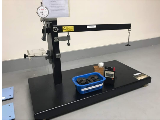
Figure 3. The set up of the creep testing machine
