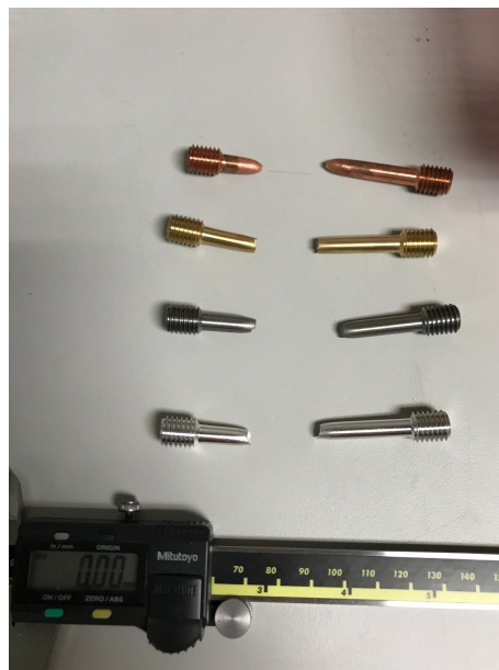
Figure 2 : Digital Vernier Caliper and 4 testing samples (Copper, Brass, Steel, Aluminium) used in experiment
