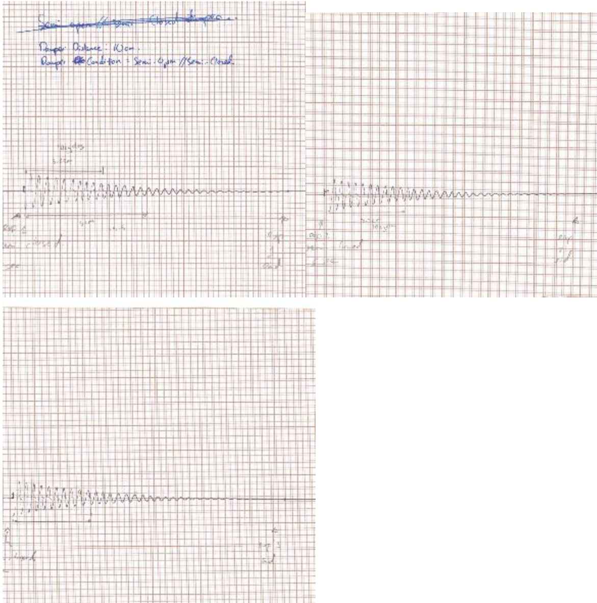
Figure 13: Spring 3, Semi-closed Damper, 10cm Distance, 3 Iterations
