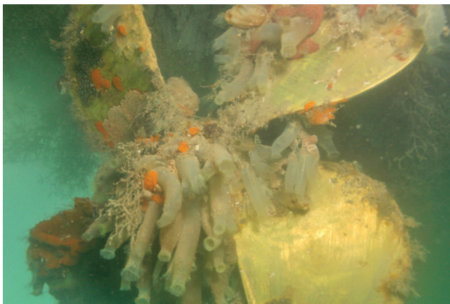
Figure 5 Propeller of a domestic vessel fouled by the invasive ascidian, Ciona robusta . Longer-term strategies for reducing invasion risk include the implementation of widely-adopted, best-practice hull maintenance regimes that reduce fouling. (Photo: Javier Atalah, Cawthron Institute)
