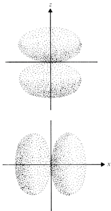
Figure 2.5 The spatial configurations of p orbitals.
