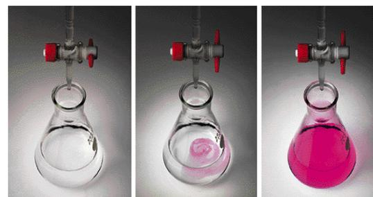
Mechanism for phenolphthalein indicator. At Low pH phenolphthalein is colorless and has a structure in which there is a five membered ring. In the presence of excess acid the five membered ring is broken and the resulting change in conformation gives rise to a compound which is pink.
