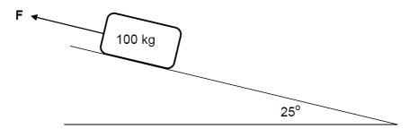
The magnitude of the kinetic frictional force  $(f_k)$  between the block and the surface of the inclined plane is 266 N.
