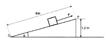
4.1 Draw a labelled, free-body diagram showing all the forces acting on the box as it slides down the inclined plane.
