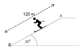
The total kinetic friction between the skis and the slope was 150 N between points  ${\bf A}$  and  ${\bf B}$ .
