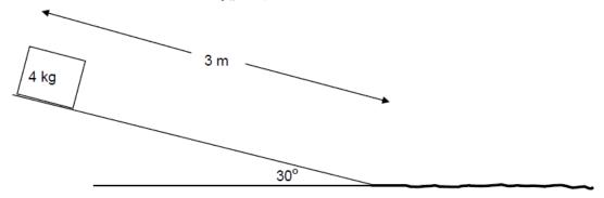
At the bottom of the plane, the mass slides along a rough horizontal surface with a coefficient of kinetic friction 0,5 until it comes to rest.
