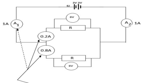
Parallel resistors divide the current (I) proportionally, so: the bigger the resistor, the lower the current flow; the smaller the resistor, the bigger the current flow,
