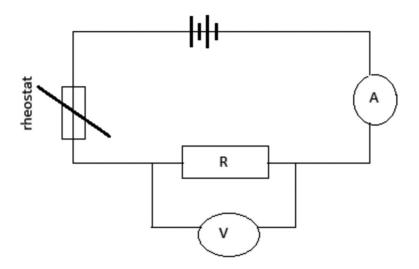
The rheostat is used to vary the current by increasing or decreasing the resistance, i.e.changing the current of the circuit.
