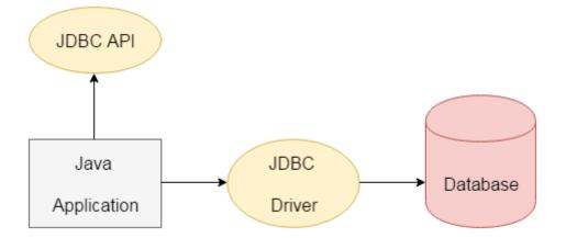
The current version of JDBC is 4.3. It is the stable release since 21st September, 2017. It is based on the X/Open SQL Call Level Interface. The **java.sql** package contains classes and interfaces for JDBC API. A list of popular *interfaces* of JDBC API are given below:
