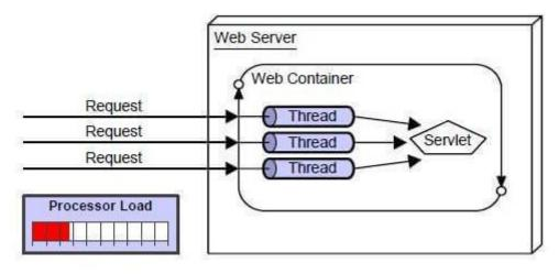
There are many advantages of Servlet over CGI. The web container creates threads for handling the multiple requests to the Servlet. Threads have many benefits over the Processes such as they share a common memory area, lightweight, cost of communication between the threads are low. The advantages of Servlet are as follows:
