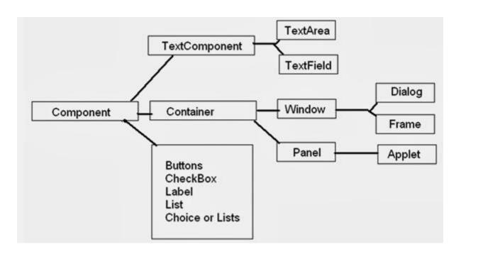
As you see this Figure this Hierarchical view display all the classes and also their Sub Classes. All the Classes are Contained as a Multi-Level inheritance, As You see that Component Class contains a Panel Class which again Contains a Applet Class so that in the AWT Package are Stored in the form of Multi-values
