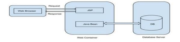
As shown in above architecture, web browser directly accesses the JSP page of web container. The JSP pages interact with the web container's JavaBeans which represent the application model. When client sends request from a JSP page, the response is sent back to the client depending on the requests which are invoked by the client request. If response requires accessing the database, the JSP page uses JavaBeans to get data from the database.
