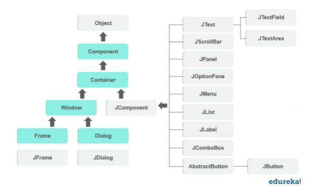
All the components in swing like JButton, JComboBox, JList, JLabel are inherited from the JComponent class which can be added to the container classes. Containers are the windows like frame and dialog boxes. Basic swing components are the building blocks of any gui application. Methods like setLayout override the default layout in each container. Containers like JFrame and JDialog can only add a
