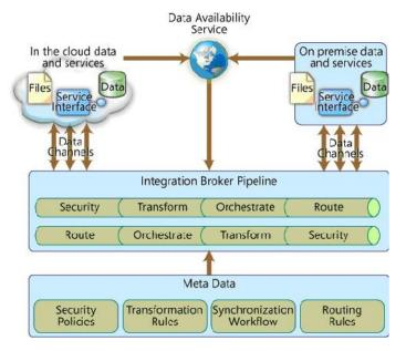
Data can originate from different sources, using different protocols and a variety of mutually incompatible formats. The job of the integration broker is to take data from a variety of
