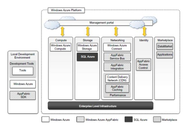
Compute services are the core components of Microsoft Windows Azure, and they are delivered by means of the abstraction of roles. A role is a runtime environment that is customized for a specific compute task. Roles are managed by the Azure operating system and instantiated on demand in order to address surges in application demand. Currently, there are three different roles: Web role, Worker role, and Virtual Machine (VM) role.
