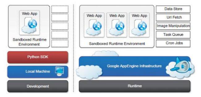
App Engine is a platform for developing scalable applications accessible through the Web. The platform is logically divided into four major components: infrastructure, the run- time environment, the underlying storage, and the set of scalable services that can be used to develop applications.
