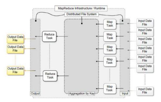
Distributed grep: The grep operation, which performs the recognition of patterns within text streams, is performed across a wide set of files. MapReduce is leveraged to provide a parallel and faster execution of this operation. In this case, the input file is a plain text file, and the map function emits a line into the output each time it recognizes the given pattern. The reduce task aggregates all the lines emitted by the map tasks into a single file.
