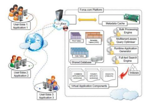
A runtime engine executes application logic by retrieving its metadata and then performing the operations on the data. Although running in isolated containers, different applications logically share the same database structure, and the runtime engine executes all of them uniformly. A full-text search engine supports the runtime engine. This allows application users to have an effective user experience despite the large amounts of data that need to be crawled.
