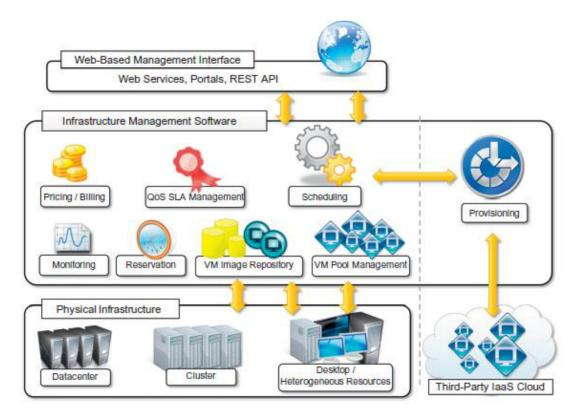
Besides the basic virtual machine management capabilities, additional services can be provided, generally including the following: SLA resource-based allocation, workload management, support for infrastructure design through advanced Webinter- faces, and the ability to integrate third-party IaaS solutions.
