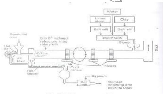
Fig. 9.1 Rotary cement kiln
