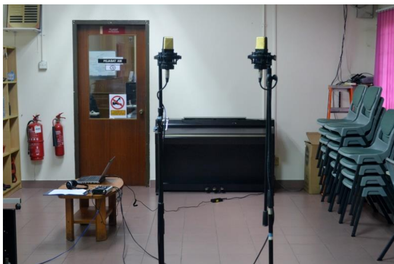
Figure 5: Placing a pair of AKG C414 condenser microphones to pick up the sine wave sweep from the loud speakers (photograph by Musib, 2017).
