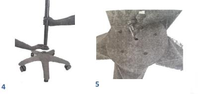
Place bottom end of Pole #1 through decorative ring and screw into wheel base.
