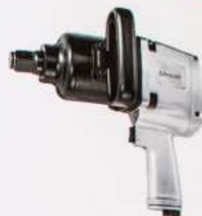
UI83P 1" Impact Wrench Pistol 1" Anvil 2440 Nm 1/2" Air Inlet
