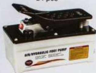
HJHM3501 Air Hydraulic Foot Pump 10,000 Psi Pressure 1600 ml Oil Capacity 11 in 3 /min Flow 1/4" Inlet 1/2" Outlet
