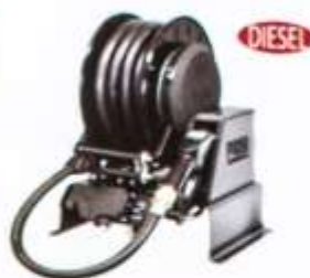
PS212000 Pitstop 1/2" 12v Hose Reel With Two Integrated Pumps 45 l/min 30 min Duty Cycle Includes: Control, 14m Hose, Cartridge Filter Lockable Saddle for Control
