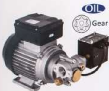
PS302040 Visco-Flomat 230 1" 220v Oil Gear Pump 14 L/min 16 Bar Auto Shutoff Adjustable By-Pass Valve
