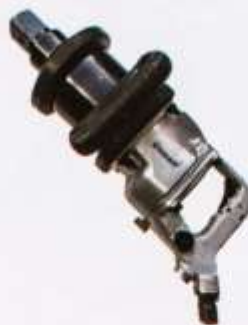
UI83 1" Impact Wrench 2" Anvil 2440 Nm 1/2" Air Inlet
