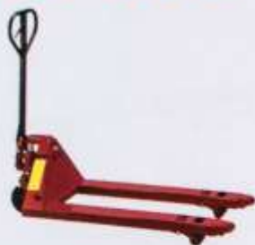
TRDF685 Hydraulic Pallet Jack Fork Outer Width - 690mm Lifting Range 80 - 180mm 2500Kg Capacity
