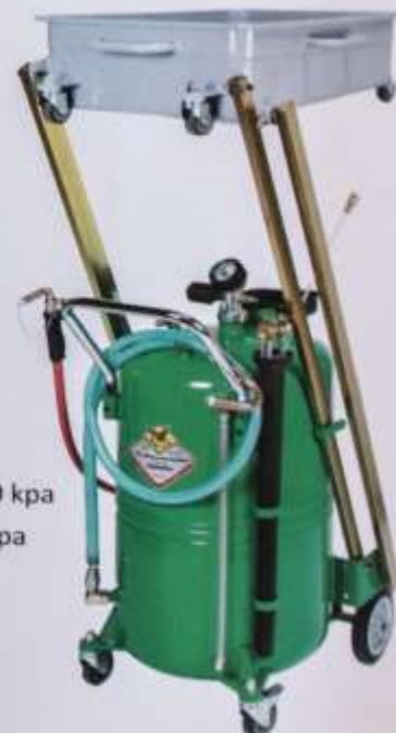
RM44084 Air Operated Waste Oil Evacuator / Drainer Tank - 80L Bowl - 16L Depressurising Pressure - 700 kpa Discharging Pressure - 50 kpa Drain Hose - 2m Suction Time - 2 U/m
