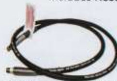
AME16105 3m High Pressure Hydraulic Hose 1/4" male x 1/2" male 10 000 Psi
