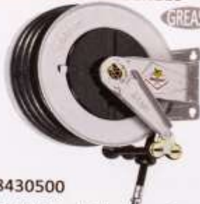
RM8450400 15m 1/2" Retractable Enclosed Hose Reel with Fixed Mounting Bracket & Hose Stop - NO HOSE Inlet : 1/2" Female Outlet : 1/2" Female Optional Hose - HOSER115
