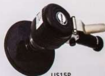
US15P 6" H/D Dual Sander 10000 RPM 1/4" Air Inlet (Stick-on Discs)
