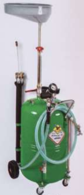
RM44084 Air Operated Waste Oil Evacuator / Drainer Tank - 80L Bowl - 16L Depressurising Pressure - 700 kpa Discharging Pressure - 50 kpa Drain Hose - 2m Suction Time - 2 U/m
