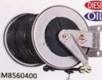
RM8530400 20m 1/2" Retractable Hose Reel with Fixed Mounting Bracket & Hose Stop - NO HOSE Inlet : 1/2" Female Outlet : 1/2" Female Optional Hose - HOSER120
