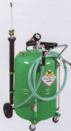
RM43084 Air Operated Waste Oil Evacuator Tank - 80L Depressurising Pressure - 700kpa Discharging Pressure - 50 kpa Drain Hose - 2m Suction Time - 2 U/m
