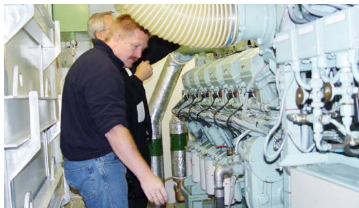
Four-stroke gas engines on board the MS GLUTRA .
