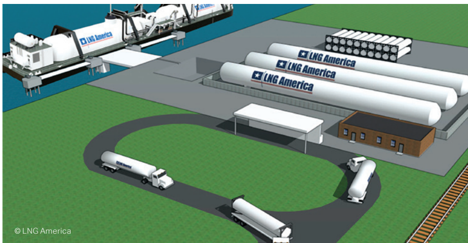
Figure 8. Marine Terminals for Loading LNG Bunker Barges, Trucks, ISO Containers and Third-party Vehicles
