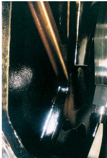
Figure 12: Taro DP (X) technology — cambox cleanliness despite 4% heavy fuel contamination
