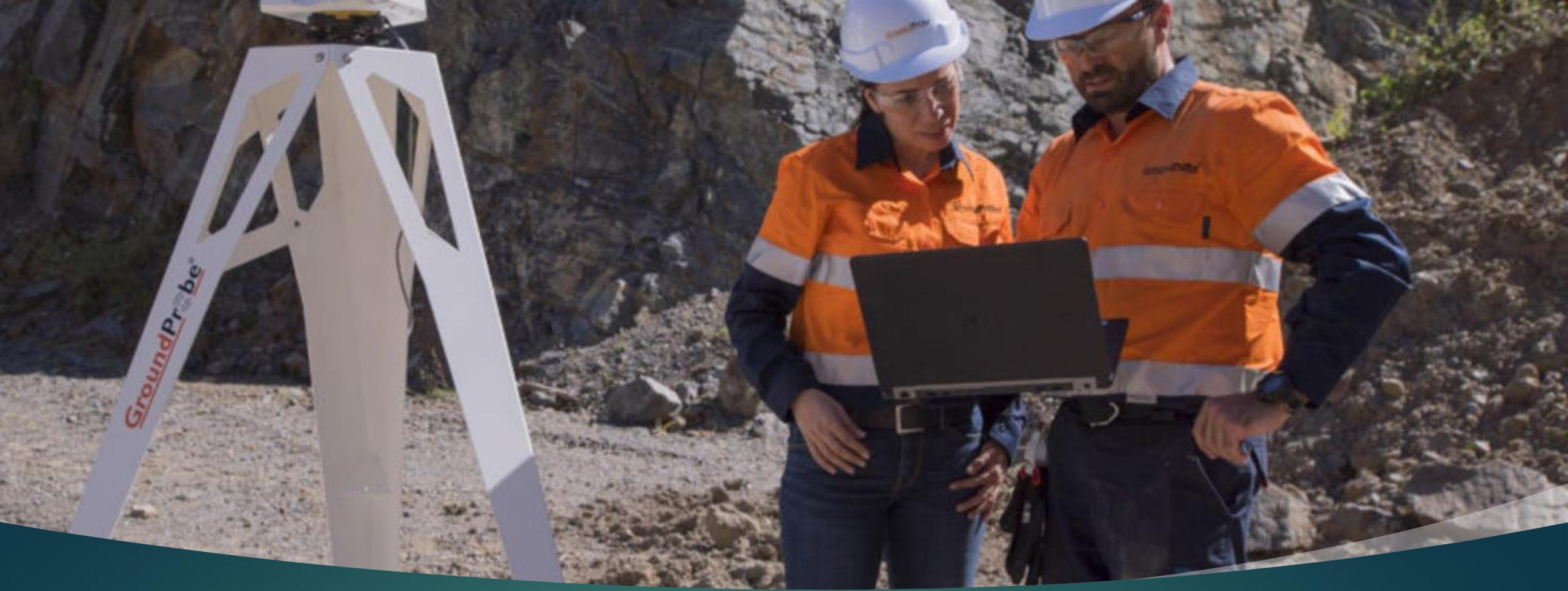
The **Geotech Monitoring Station (GMS)** replaces traditional total stations that rely on mirrored prisms to be attached to the slope. The system can scan these points, but can also reflect its signal directly off the rock without the need for prisms. It is first laser-based monitoring solution to give early warning of impending collapses of open pit mine walls, dams, mine dumps and vegetated slopes, which can begin months or years before a collapse occurs.
