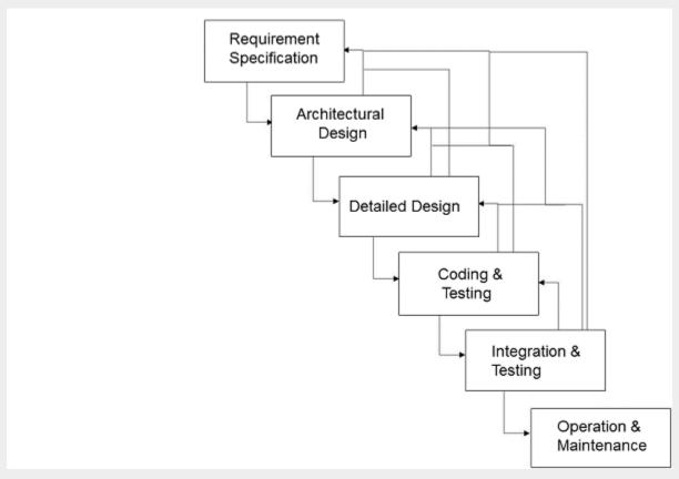
The uni-directional movement of the waterfall model of Software Engineering shows that every phase depends on the preceding phase and not vice-versa. However, this model is not suitable for the interactive system design.
