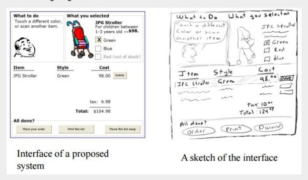
The above diagram can be considered as a **Low Fidelity Prototype** as it uses manual procedures like sketching in a paper.
