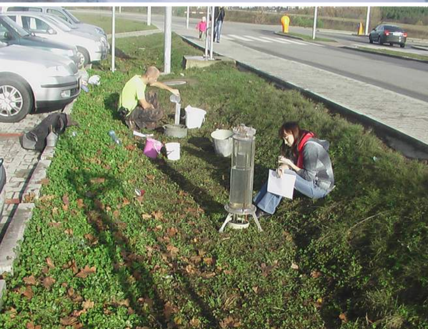
Photo 2a,b: Monitoring of the process of infiltration in the combined infiltration-retardation furrow – groove to drain precipitation water from the car park (Czech Republic, Brno, Masaryk University Campus, 2009)
