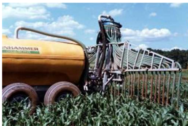
Photo 32: Application of Liquid, Stabilized and Sanitary Treated Sludge on the Soil Surface
