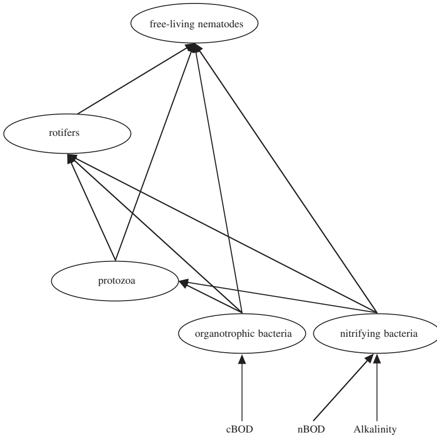
FIGURE 2.2 Transfer of carbon and energy through an activated sludge food web. Carbon and energy enter the activated sludge process in the form of cBOD and nBOD and alkalinity. These carbon and energy substrates are used by a variety of organisms in the activated sludge process, and many of the organisms that grow from these substrates in turn are used as substrates by other organisms. The transfer of carbon and energy in the activated sludge process is between many groups of organisms in a “web-like” pattern.
