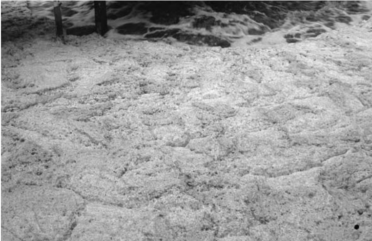
FIGURE 20.1 Foam on an aeration tank.
