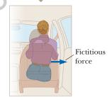
Relative to the reference frame of the Earth, the car seat applies a real force (friction) toward the left on the passenger, causing her to change direction along with the rest of the car.
