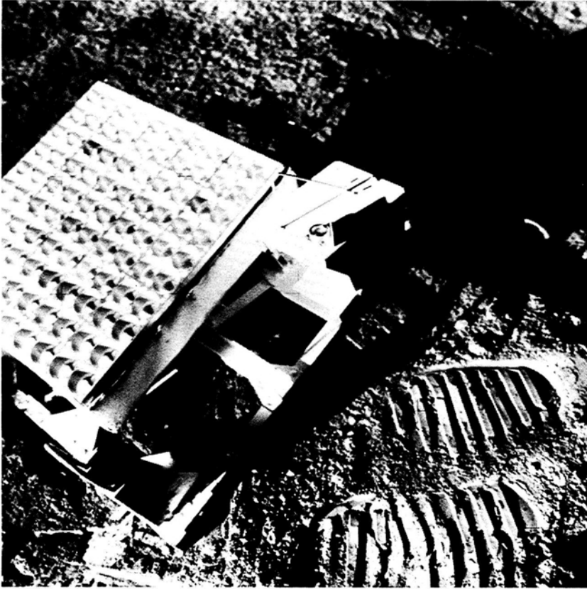
FIGURE 3.2 The array of corner reflectors placed on the Moon by Apollo 14 astronauts (note footprints). The bubble level and gnomon, used for pointing the array toward the Earth, can be seen. Laser range measurements are routinely made to three widely separated arrays. No degradation of their optical reflectivity has been observed.
