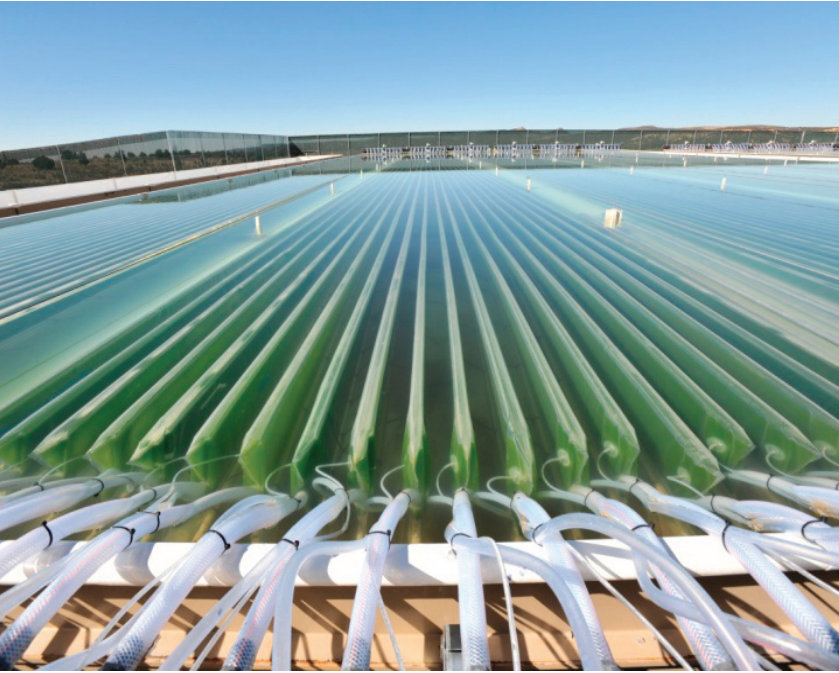
FIGURE 2-9 Solix photobioreactor. SOURCE: Reprinted with permission from Solix Biosystems.
