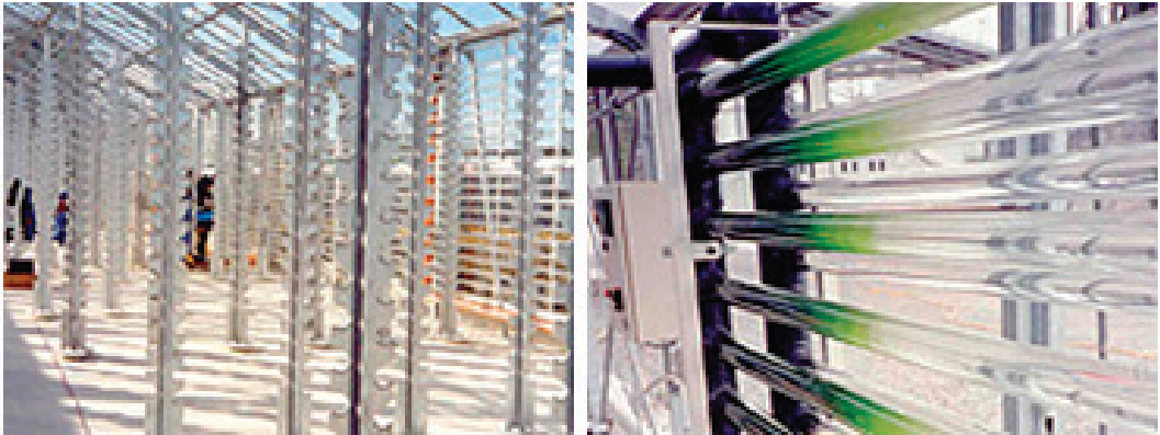
FIGURE 2-7 Tubular photobioreactors of straight horizontal tubes stacked in vertical fence-like arrays housed in a greenhouse in Klotze, Germany. SOURCE: Algomed. Reprinted with permission from AGU.
