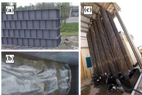
Fig. 19.6 a–b Converting aeration tank to MFC by submerging electrodes inside (advanced environmental technologies, USA). c Tubular MFC system for brewery wastewater treatment and electricity/caustic production (U of Queensland, AU)
