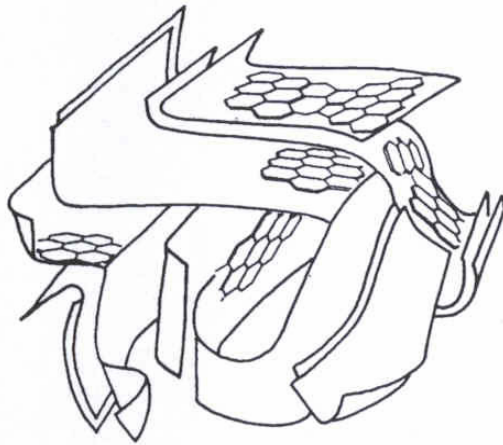
Fig.3.2: A schematic representation of the structure of activated carbon. Adapted from Stoeckli (1990) (Courtesy of Elsevier).
