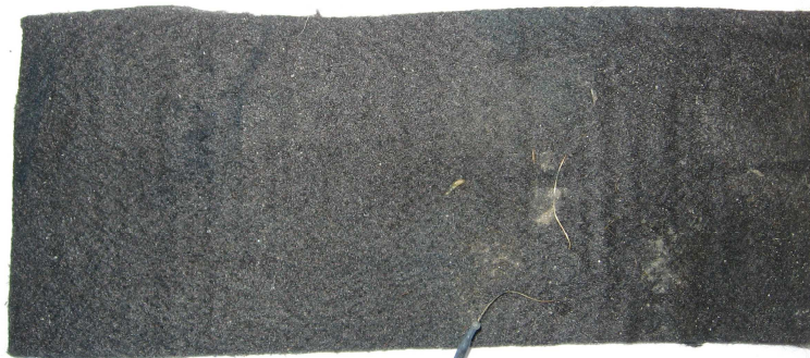
Figure 6.5: Picture of the graphite felt of the setup after dismantling of the PMFC 2. The picture shows that the graphite felt was not well penetrated by plant roots.
