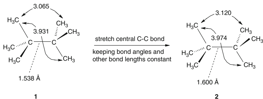
Fig. 3.8 Structures for a simple MM “by hand” calculation on the effect of changing the central C–C length of (\text{CH}_3)_3\text{C}-\text{C}(\text{CH}_3)_3 from 1.538 Å to 1.600 Å
