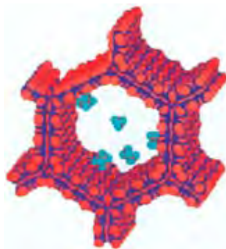
FIGURE 7.21(b) Computer graphic of ethane and methane molecules inside one of the hexagonal pores of MCM-41.
