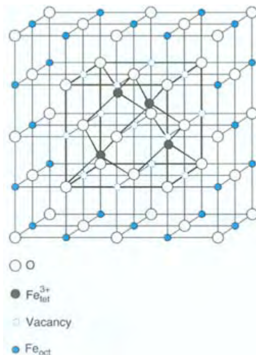
FIGURE 5.26 The Koch-Cohen cluster illustrated with the back and front planes cut away for clarity. The central section with four tetrahedrally coordinated \text{Fe}^{3+} ions is picked out in bold.
