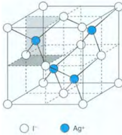
FIGURE 5.43 The zinc blende structure of \gamma -AgI.
