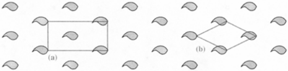
FIGURE 1.18 Choice of unit cell in a centred-rectangular lattice.
