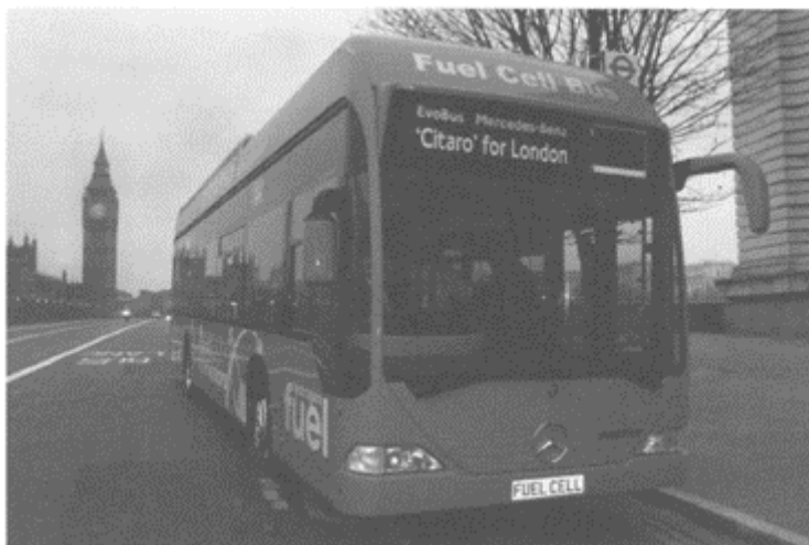
FIGURE 5.19 A zero-emission Mercedes Citaro bus operating in London, powered by a Ballard ® fuel-cell engine. (Courtesy of Ballard Power Systems.)
