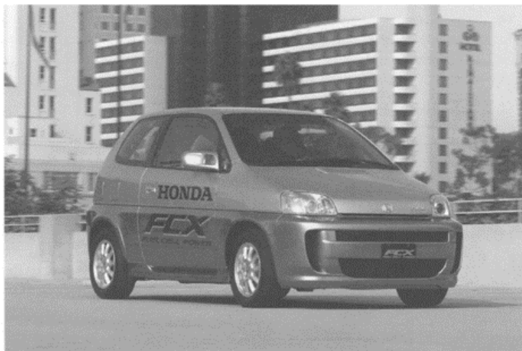
FIGURE 5.21 Honda Motor Company's hydrogen-fuelled FCX fuel-cell car with a range of 170 miles and a top speed of 93 mph. (Courtesy of Ballard Power Systems.)
