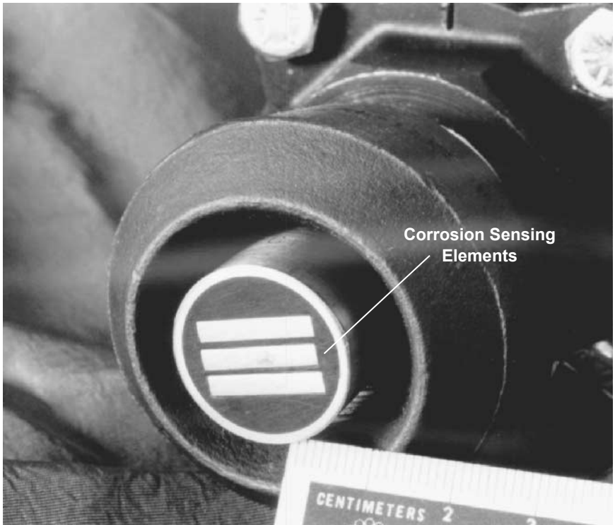
Figure 6.26 Close-up of corrosion sensing elements used for thin-film corrosion monitoring.
