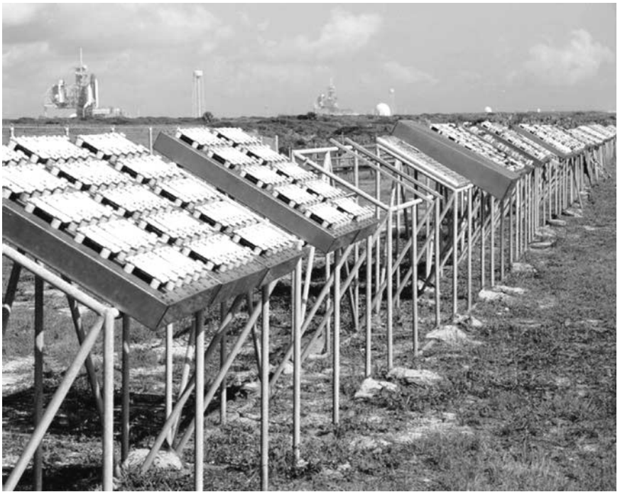
Figure 7.41 Ground view of the Kennedy Space Center beach corrosion test site with a background view of the Shuttle.
