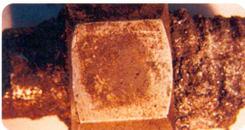
Corroded bolt from galvanic corrosion. From Stress-Corrosion Cracking and Galvanic Corrosion of Internal Bolts from a Multistage Water Injection Pump , J. of Failure Analysis and Prevention, Vol 8, No. 1, p 48-53, 2008.
