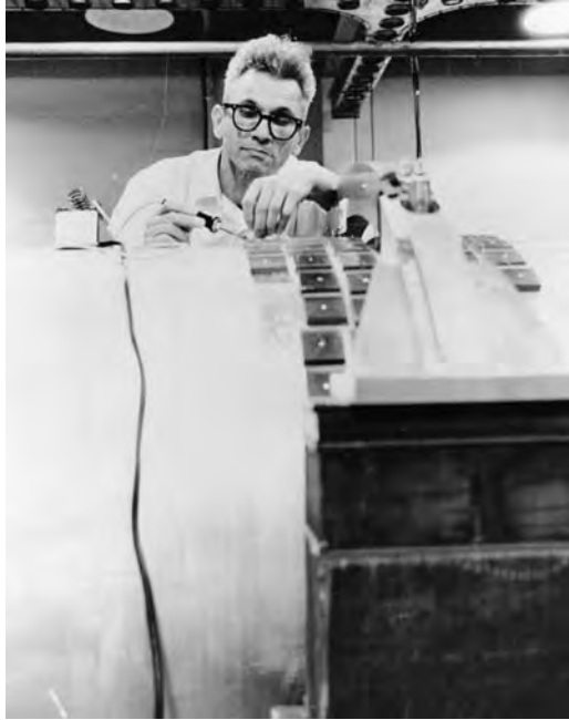
Figure 2.7 Joseph Weber working on a bar detector at the University of Maryland in the early 1970's. The fundamental frequency of the bar was 1660 Hz. Piezoelectric crystals around the center of the bar convert tiny mechanical vibrations to electrical signals. (Courtesy of AIP Emilio Segre Visual Archives)
