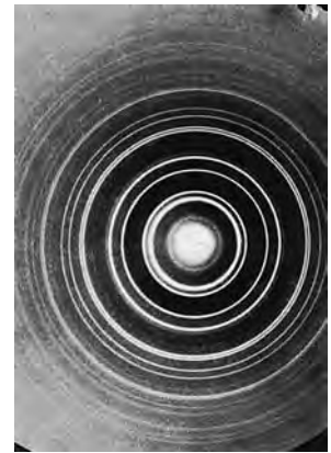
Figure 5.7 Diffraction of 50-kV electrons from a film of \text{Cu}_3\text{Au} . The alloy film was 400 \text{ \AA} thick. (Courtesy of the late Dr. L. H. Germer)
