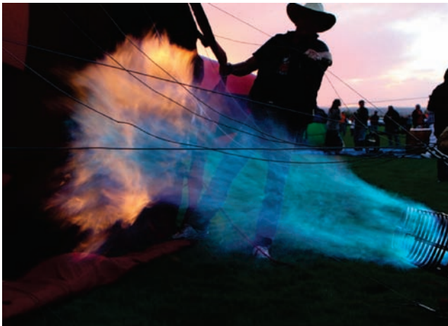
Figure 6.2 Propane flame with slightly luminous tail, indicating some soot formation and corresponding increase in flame emissivity.
