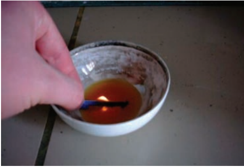
Figure 3.22 This liquid is too cold, the flash point is not reached.
