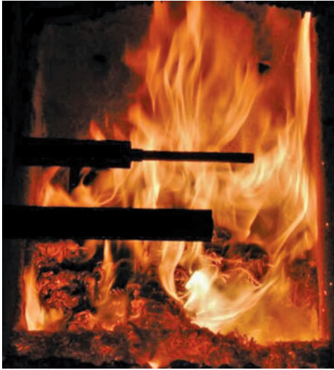
Figure 5.46 A temperature probe and a cooled suction probe in the pilot plant of the Institute of Combustion and Power Plant Technology, University of Stuttgart/Germany [125].
