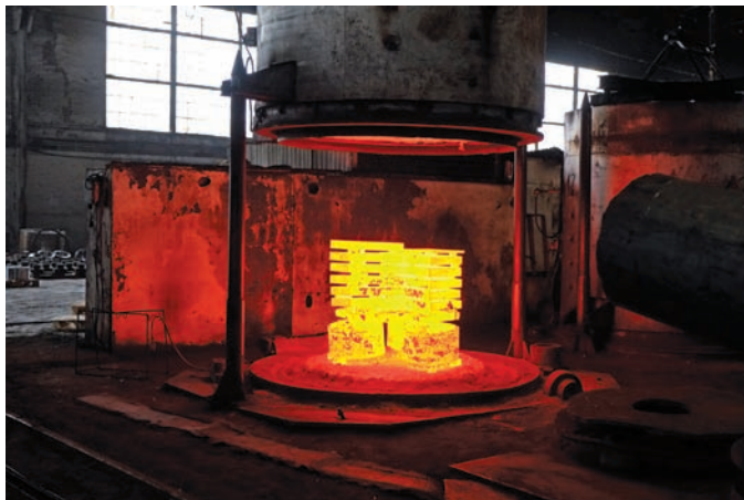
Figure 6.24 Bell furnace with raised bell and glowing hot batch inside.
