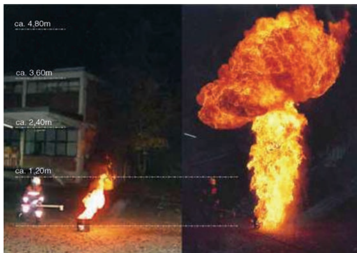
Figure 7.4 Water is not a suitable fire extinguishing agent for burning oil. As the burning oil has a high temperature, typically 300–350 °C, the water will instantly vaporize and disperse the oil into droplets with a very large surface area, leading to a huge fireball [3].
