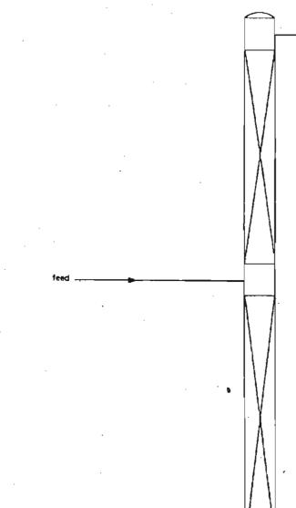
Figure 2a Basic symbol for fluid contacting device applied to a packed column used for distillation of a twocomponent mixture into two fractions
