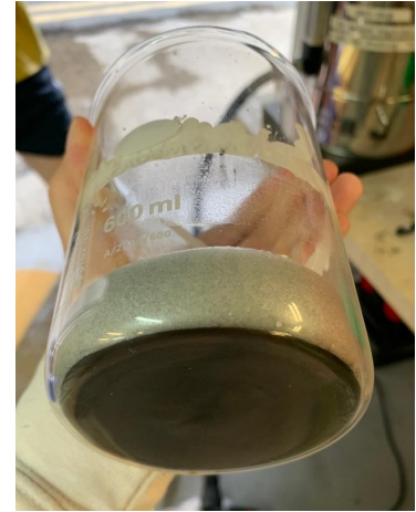
Figure 3.2: The PCM-graphite mixture when solid, showing the accumulation of graphite at the bottom of the container.
