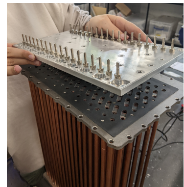
Figure 2.11: The front manifold plate being attached to the front pipe plate, with the silicone gasket in between.
