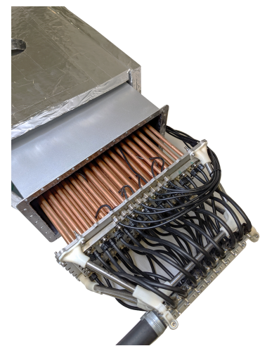
Figure 1.2: The PCM unit in a partially assembled state, showing the insulation, container and heat exchanger.
