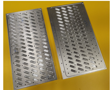
Figure 2.2: The rear of the manifold plates, showing the return-bend slots.
