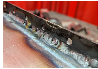
Figure 2.14: A badly contaminated TIG weld, which caused the PCM container to leak.
