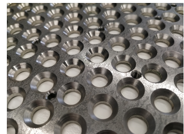
Figure 2.6: Chamfered holes on the pipe plates, to guide the flow of solder during brazing.
