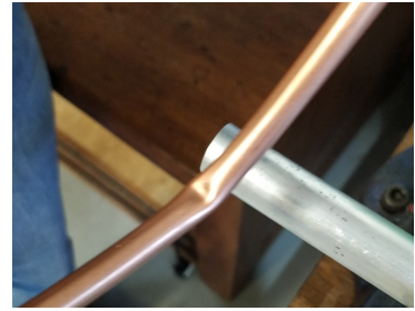
Figure 2.1: The unsuccessful result of an early pipe bending test.
