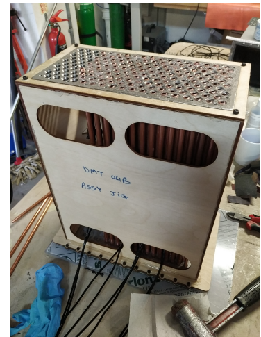
Figure 2.8: The plywood assembly jig holding the pipe plates in place while the copper pipes were glued into place.
