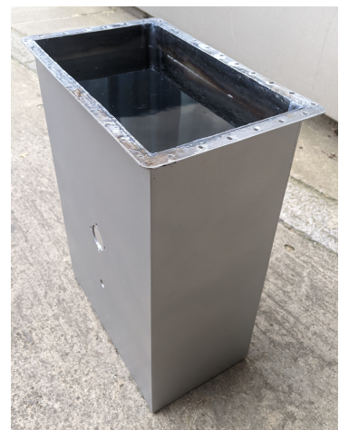
Figure 2.15: The PCM container, having been painted and sealed with epoxy, filled with water for a leak test.
