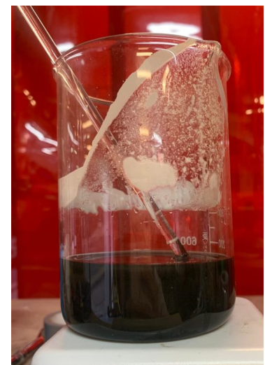
Figure 3.1: The PCM-graphite mixture when liquid.
