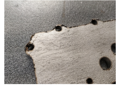
Figure 2.4: Poor results from laser cutting
