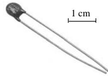
Figure 8.1 Thermistance. *Transistek*
