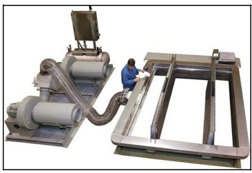
Shop test of the a FGD Tandem seal damper. The damper was later installed in Cyprus.
