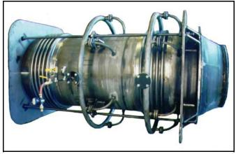
Ø40 inch diameter Universal refractory lined expansion joint for Styrene Monomer service. Two ply Inco 800HT monitored bellows with purged liners. –15 to 29 psig at 1202°F.
