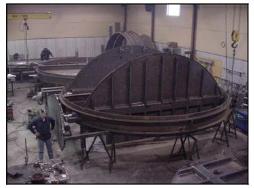
HRSG Stack Damper for a GE 7F in the United States being shop tested
