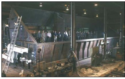
SCR Diverter (9 foot 6 inch wide by 66 foot 10 inch flap) with more than 20 workers standing on the flap. This diverter was later shipped and placed into service in the United States
