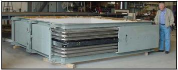
120 inch square hinged refractory lined universal expansion joint for a refinery. Inco 600 bellows with rounded corners. 2 psig at 1200°F.
