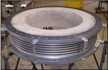
Ø82-1/2 inch diameter single refractory lined expansion joint for steel mill hot blast main. Inco 600 bellows with 12 inch thick refractory. 50 psig at 1900°F.
