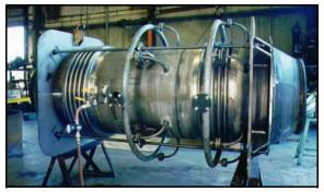
Pressure Testing of Bachmann Metal Expansion Joint
